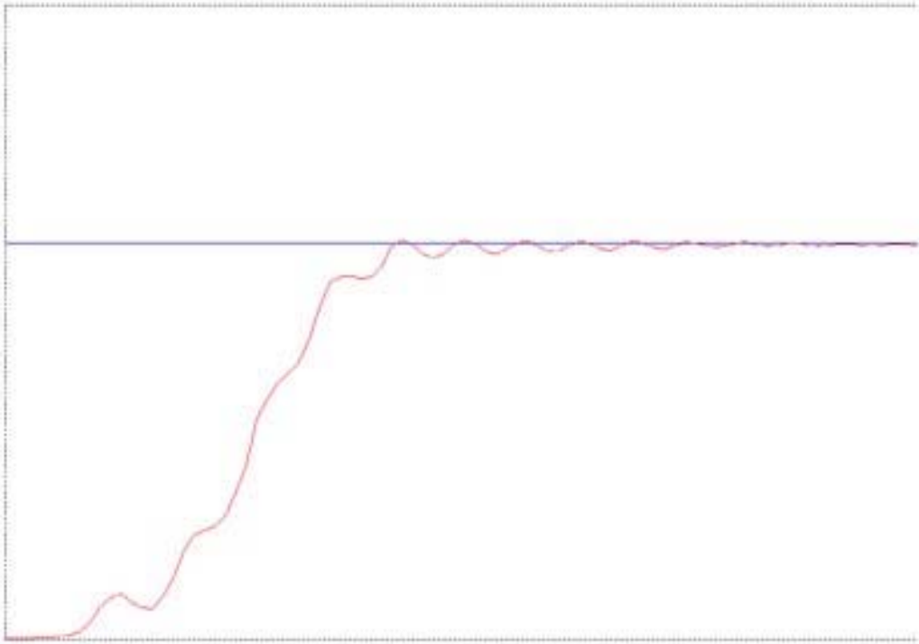
Step function response with K_p too high
