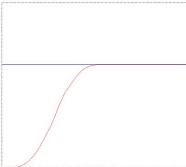
Ideal system response to a step function
