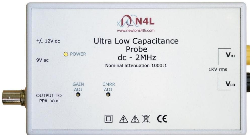
Accessory for use with the PPA range power analyzer in applications where capacitance to ground must be minimized.
